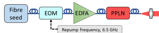
FIG. 9. Schematic of the laser used for optical trapping. The output light from a seed laser (1550 nm) is modulated by an EOM driven by a 6.5 GHz oscillator to generate frequency sidebands. The light is then amplified by an EDFA before being frequency doubled via second harmonic generation using a PPLN waveguide. The output of the fiber is allowed to expand, before being collimated using a lens. This collimated light is then input into the MOT vacuum chamber.
