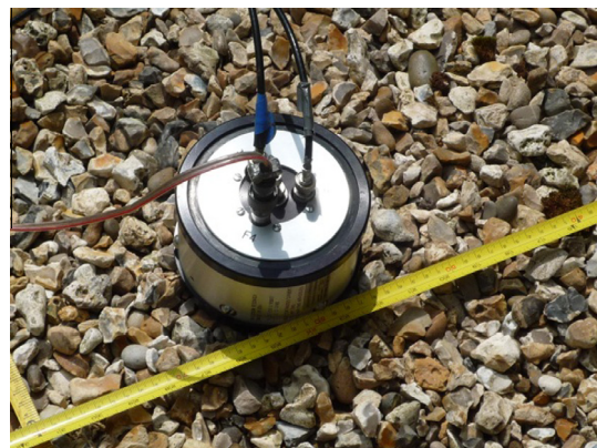
Fig. 5. Electrodynamic shaker (here on a gravel surface).
