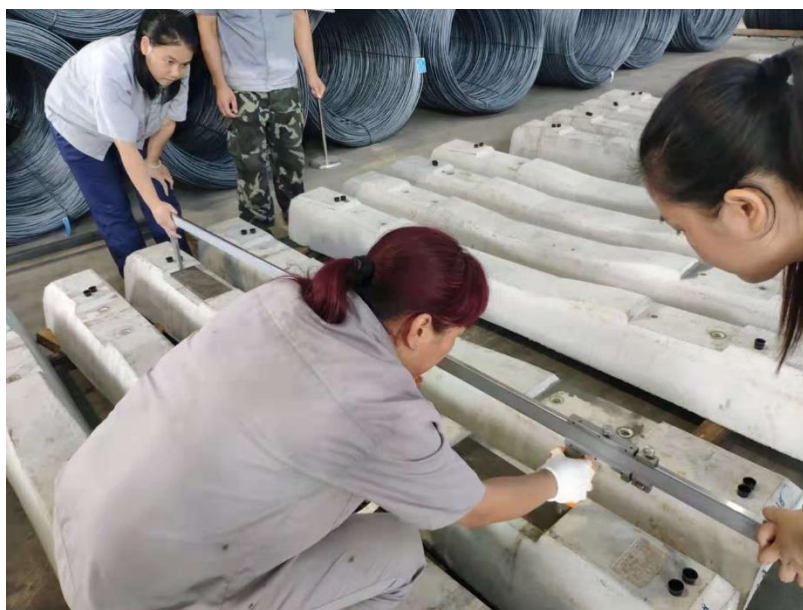
Figure 9. Sleeper critical dimension measurement
