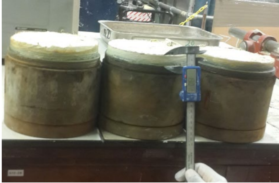
Figure 5 Swelled soil specimens after a 11 month period in a water tank
