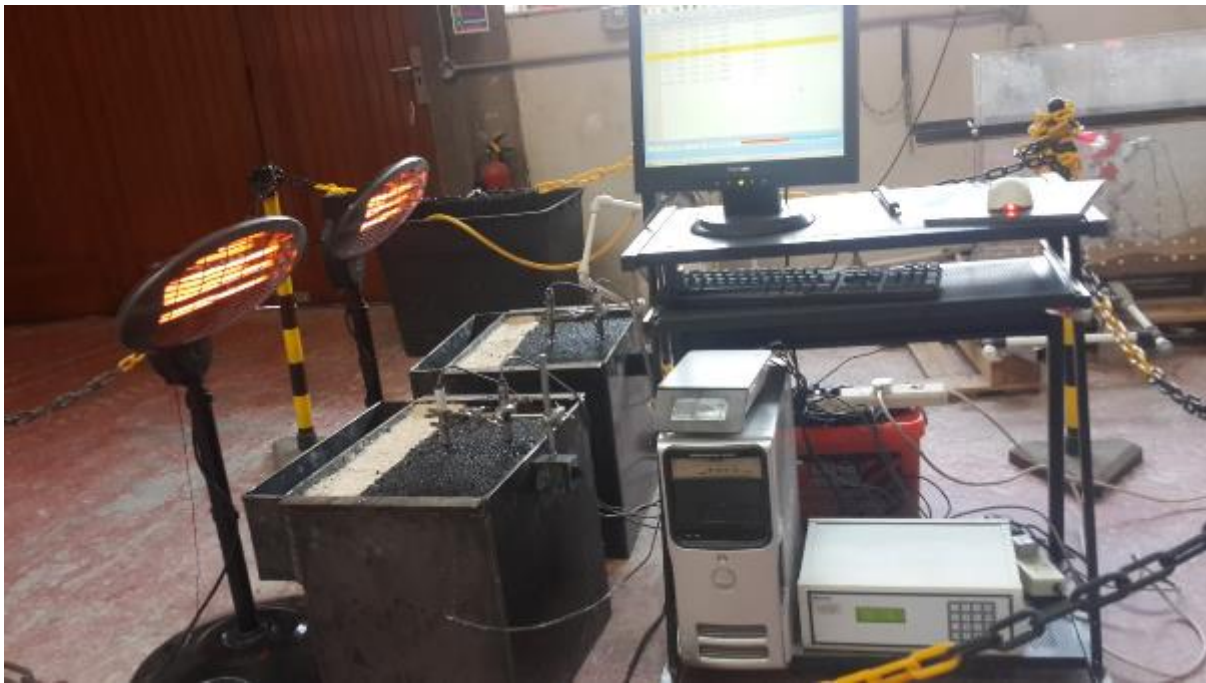
Figure 3 Test in progress where drying period is being simulated by infrared heaters
