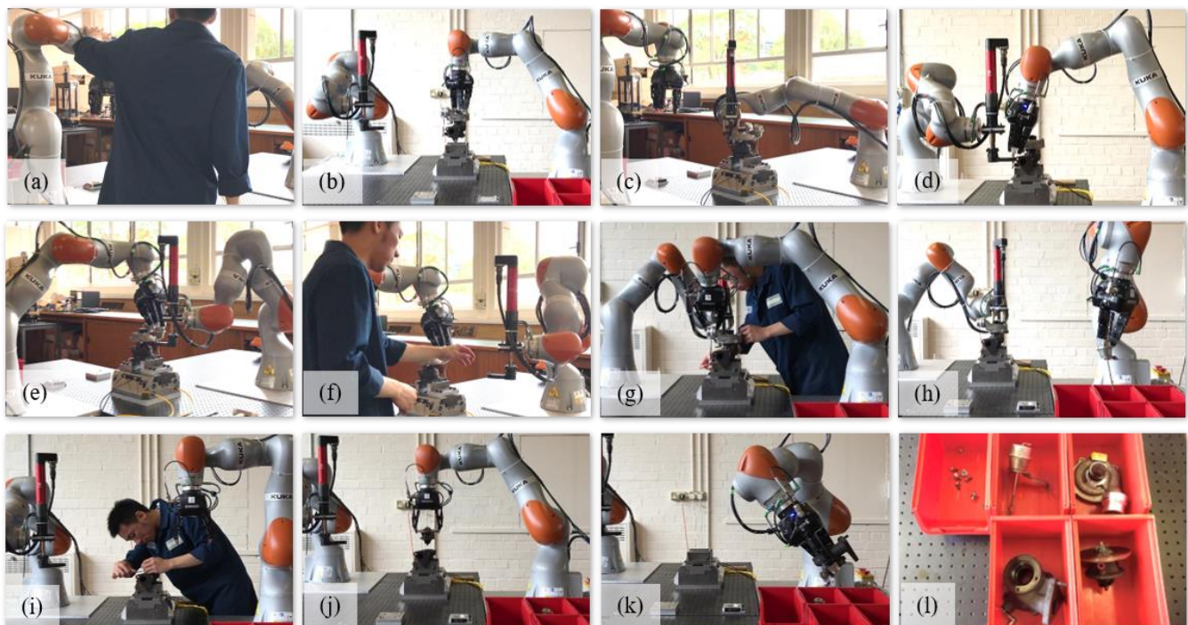
Fig. 10. Photographs of the disassembly process: (a) force control to task T1, (b)-(k) the process and (l) the dismantled parts in containers.
