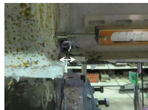
Bare specimen at 3.0% story drift: 40 mm separation of the bottom flange from the diaphragm edge
