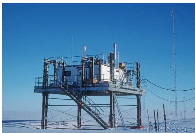
Fig. 3. The Clean Air Sector Laboratory (CASLab) at Halley. In the background is the 30 m mast for boundary layer meteorology experiments.
