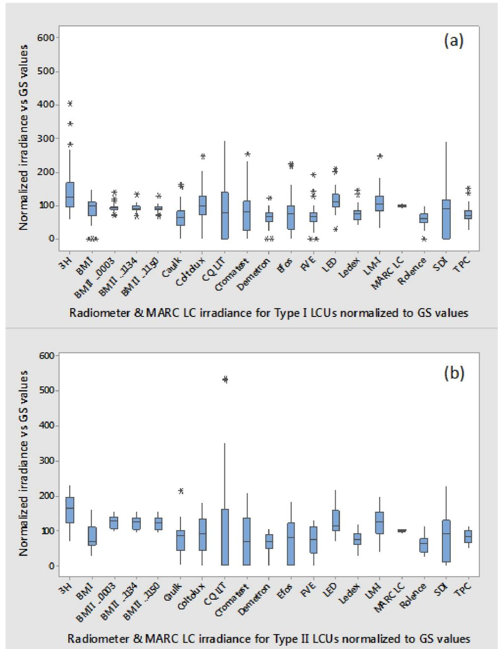
**Fig 4.** Normalized pooled mean irradiance for all LCUs; (a) Type I and (b) Type II tested with the sixteen models of dental radiometers—the 3 examples of the BM II are denoted by the last 4 digits of their respective serial numbers . . . .0003, . . . .1134, . . . .1150 and the MARC LC instrument (calculated from mean power data) relative to the gold standard Integrating Sphere method. Note the extremely wide data spread for many radiometers.
