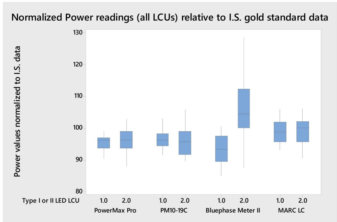
**Fig 2. Pooled normalized mean power readings for all LED-LCUs relative to the integrating sphere gold standard data 100% values.** Note the difference between the Type I and Type II LED-LCU data distributions for the BM II units (average of the three tested units shown) compared with the two laboratory-grade power meter instruments and the MARC LC integrating sphere / spectrometer apparatus.
