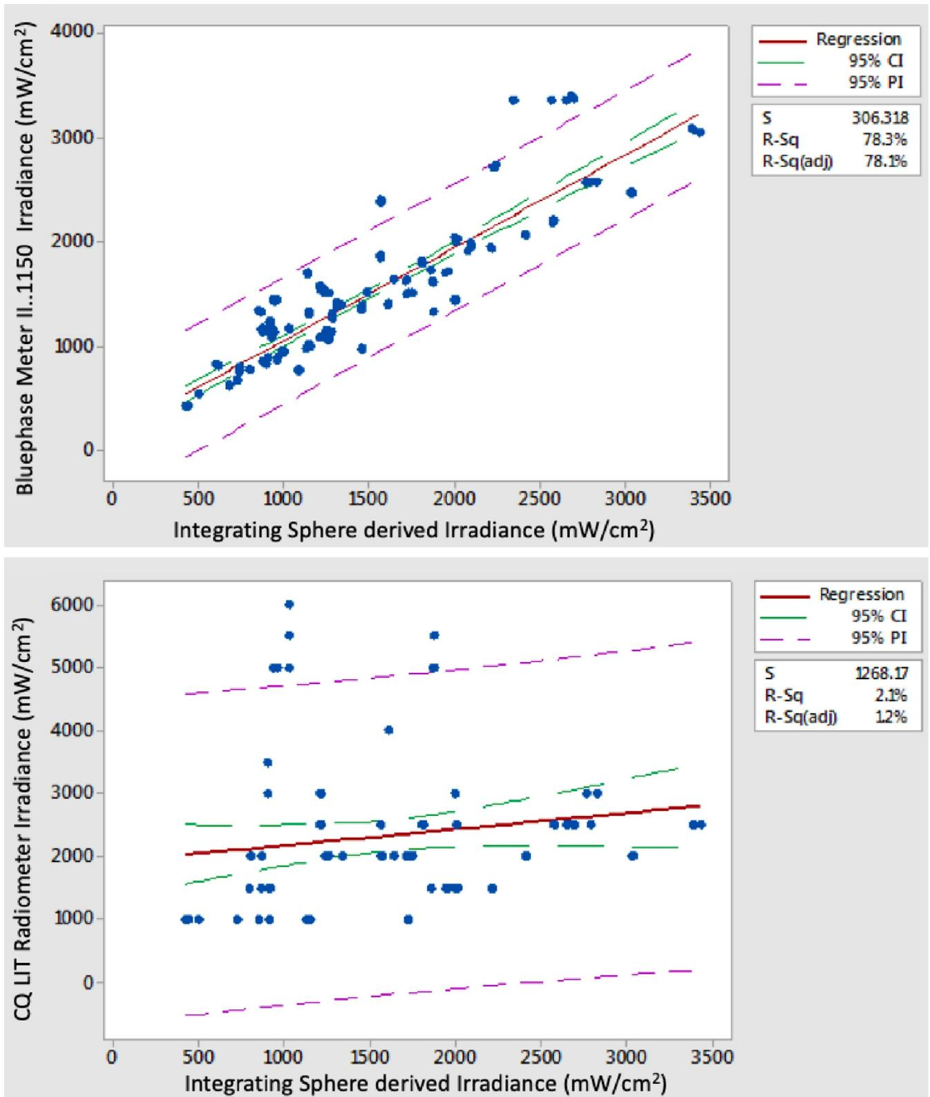
**Fig 3.** Regression analysis fitted line plots comparing irradiance data for the (a) BMII (sn:1300001150) and (b) the CQ LIT radiometer with the corresponding Integrating Sphere derived irradiance data sets as the independent variable.
