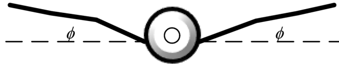
Fig 4. Auxiliary diagram of the flapping motion with the definition of the flapping angle. View in the direction of the flow.
