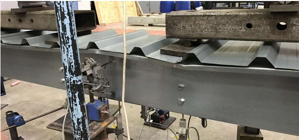
Fig.12: Failure mode of Z24615 - distortional buckling and interaction with local buckling of lip.
