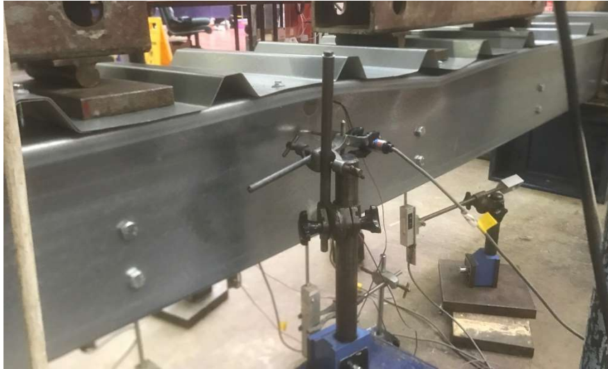
Fig.13: Failure mode of Z24620 - distortional buckling.
