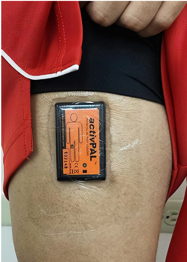
FIGURE 1 The activPAL v1 affixed to a participant's thigh using the 24-hour waterproof attachment method
