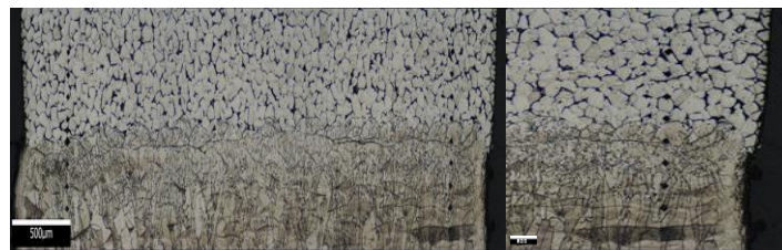
Figure 12: An image of the MIM/PBF interface after heat treatment by electro etching of specimen 1-3.
