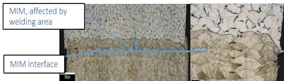
Figure 13: An image of the MIM/PBF interface without heat treatment after electro etching of specimen 1-19.
