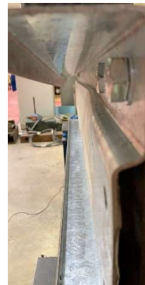
Fig. 6. Web crippling at the whole upper and middle web (a) followed by upper web twist (b) (26525-100)
