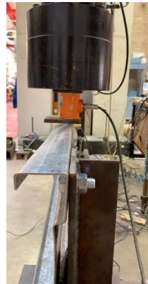
Fig. 6. Web crippling at the whole upper and middle web (a) followed by upper web twist (b) (26525-100)
