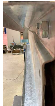
Fig. 6. Web crippling at the whole upper and middle web (a) followed by upper web twist (b) (26525-100)
