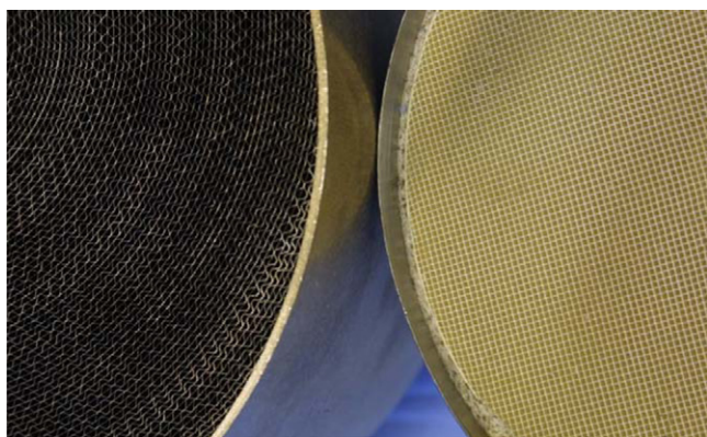
Fig. 1. Examples of metal-based catalyst (left) and ceramic-based cordierite catalyst (right).
