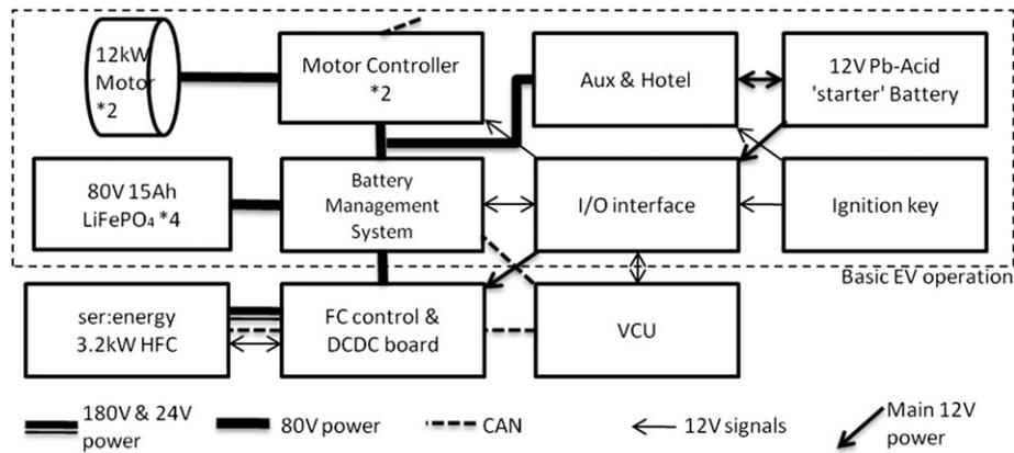
**Fig. 3.** The system architecture detailing main power flows and lines of communication, with explanations of individual systems given in the text: Sub-systems visible include the Serenergy fuel cell with its controller, the battery with its controller and the two Lynch motors with controllers.
